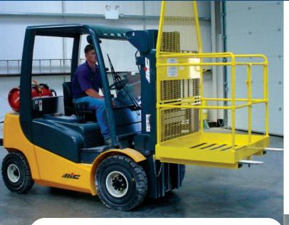
requirements of the Machinery Directive. This means that non-integrated working platforms do not meet the Supply of Machinery (Safety) Regulations. As there is no free trade in Europe for non-integrated working platforms, any used must not carry a CE mark.
